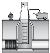
1) Install plug to isolateb manhole
