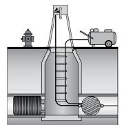
Attach Jet-Ball<sup>™</sup> to tag line and inflate
