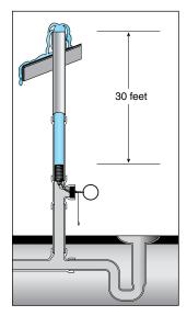
In the example above, the answer is: 30 feet of pipe above the plug = 30 feet of head
