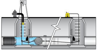
Introduce water into manhole and slowly release Jet-Ball<sup>™</sup> down the line.
