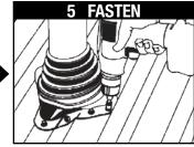
Use fasteners to complete sealing. For UPC installation, fastener spooning may not exceed 1-1/2" (38 mm).
