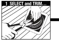
Choose appropriate Master Flash with opening at least 20% smaller than pipe diameter. If necessary trim opening to 20% smaller than pipe diameter.
