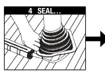
Apply sealant between base and roof.
