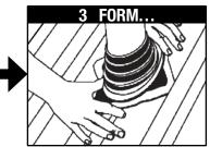
Press Master Flash down, bending it to conform to roof profile or roof irregularities. A blunt tool will help press flashing into tight roof angles.
